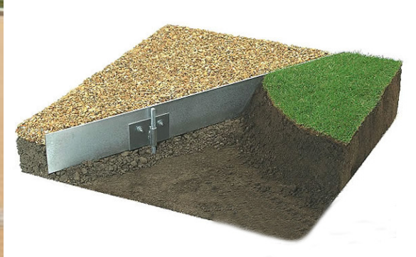
POROUS RESIN BOUND PAVING WITH STEEL EDGE TO ACHIVE CURVES
